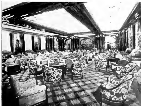
Ceiling lighting in the grand salon of the French liner Ile de France is produced from ceiling coves located in three large panels, those in the central panel being arranged as shown in the plan and section.
